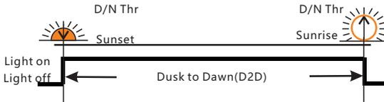
If time is set to 'D2D', the controller works in dusk to dawn mode.
